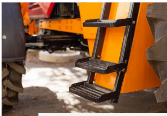
Figure 3. Non-slip footing to prevent slips, trips, and falls when accessing equipment.
